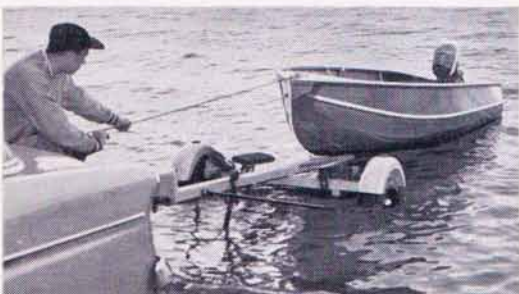
To bring boat out of water, fasten winch rope to bow, line up boat with the trailer boom and reel in the boat
