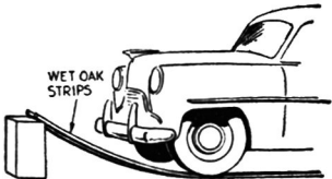
HOW TO BEND BOTTOM FRAME STRIPS
