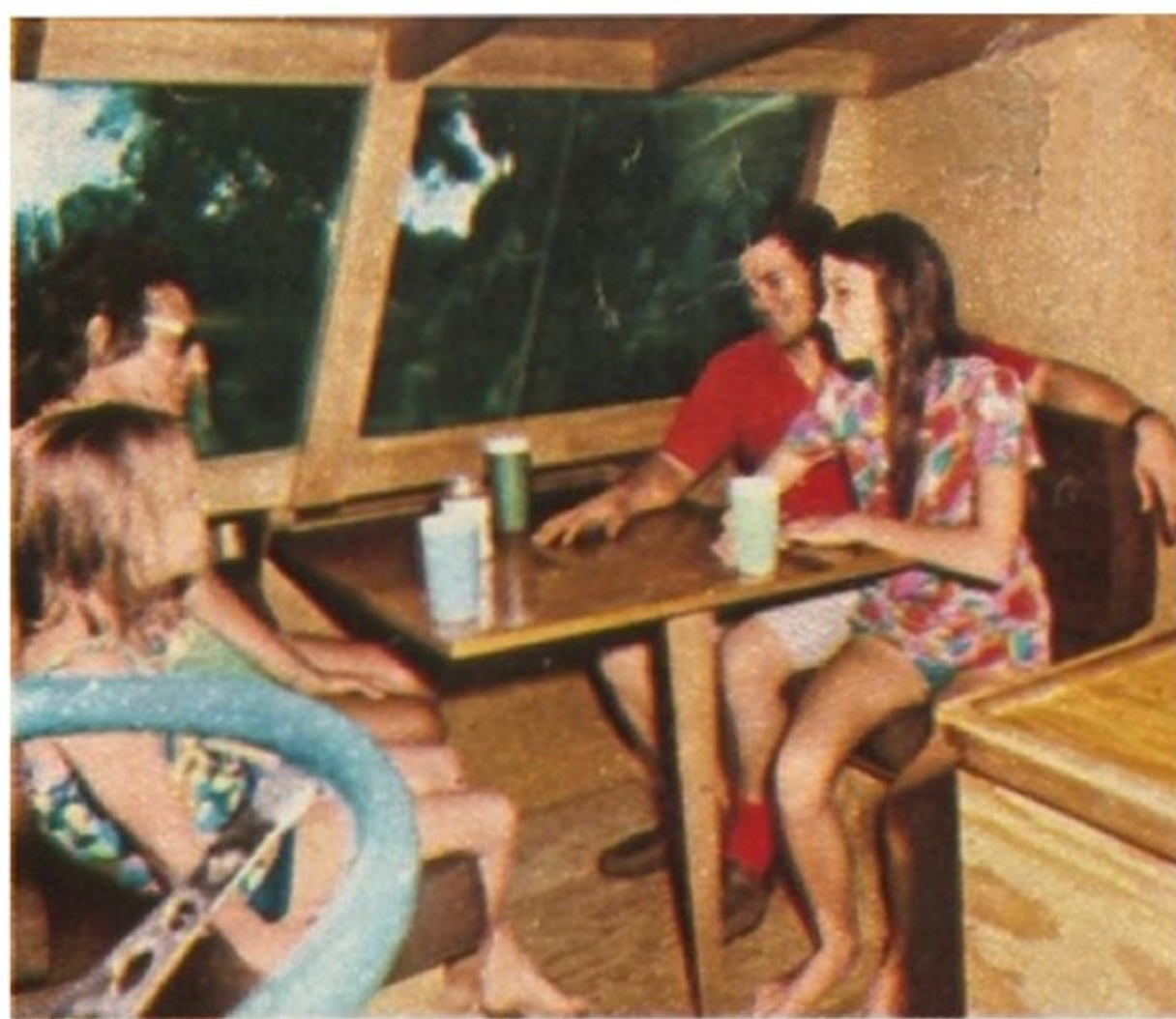
DINING table seats four, then drops flush with seats to form an extra bunk inside.
