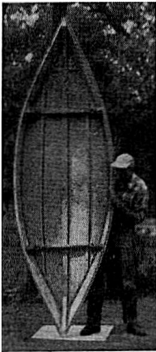
Fig. 4. Hull with bottom complete removed from form.
