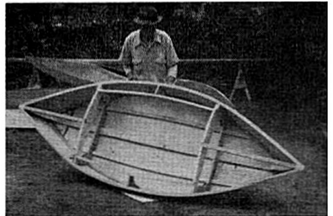
Fig. 7. Deck beams, carlins, side cockpit knee and deck battens in place.
